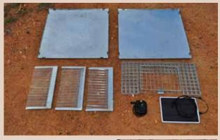
Construct the metal cage first, comprising the solid roof and floor, 3 one-way finger doors, one mesh 'rear' door for emptying the trap, and a hook on the underside of the lid to hold the light and sound attractor unit.
