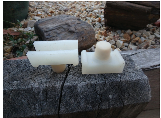
Fig. 1. Two elastomer lethal-trap devices (LTDs), each showing a nipple filled with a para-aminopropiophenone (PAPP) formulation.
