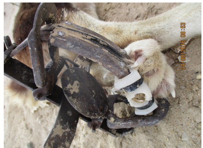
Fig. 2. A Victor ® soft catch trap (see text), with the nipple from an elastomer lethal-trap device (LTD) successfully removed by a trapped wild dog. Note the LTD is fitted to the lazy jaw (not the jaw attached to the springs) so that it faces down when the trap is set.
