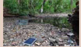
5 Ensure the trap is shaded but the solar panel is receiving sunlight by utilising the long cable supplied. Place water dripper bottle (supplied) onto the cage.
